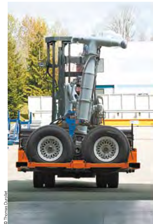
A complete landing gear being trucked to the Boeing final assembly plant.
