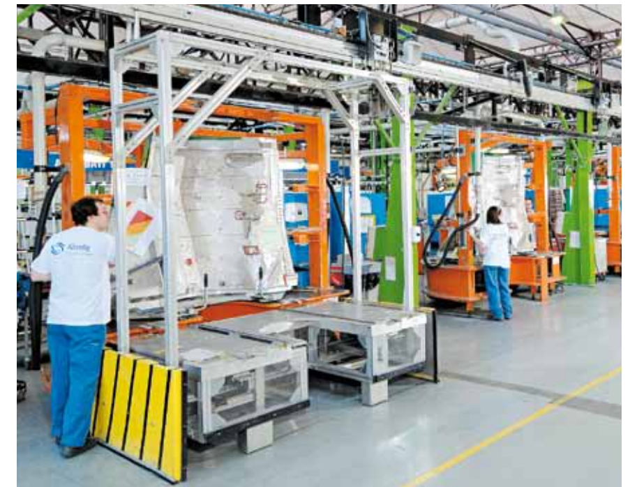
One example of how Safran Conseil supports the implementation of a Lean manufacturing approach: the reorganization of the thrust reverser assembly shop at Aircelle. The shop is shifting from separate workstations to a line approach built around the Takt time principle, which can be defined as the maximum time allowed to produce a product in order to meet demand (so that the pace of production is synchronized with the pace of delivery to customers).
