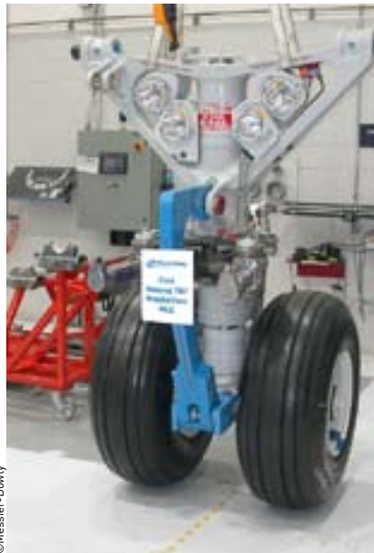
The first landing gear produced by Messier-Dowty for the 787.
